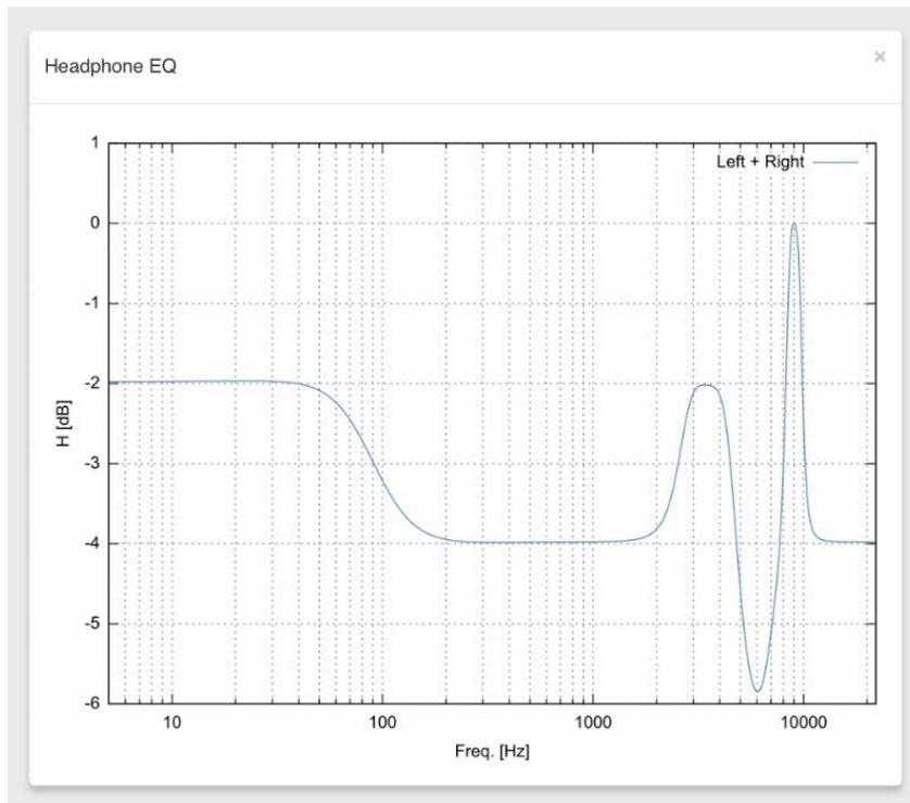
This graph shows an example of the frequency response compensation equalizer provided by Audeze.
